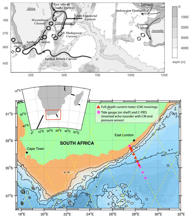
Figure 1(a) Schematic of currents in Southern Indian Ocean. Notice Agulhas Current and its leakage into the Southeast Atlantic via Agulhas Rings [9]. (b) Position of the ACT array across the Agulhas. TOPEX/Jason altimeter ground track is shown in yellow dashed lines. Inset map shows positions of other observing arrays in the region. Bathymetry contours every 1 km.
