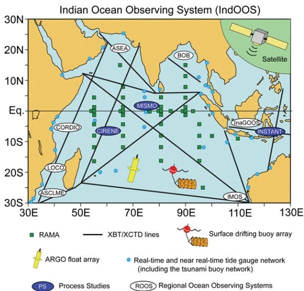
Figure 1. Schematic of the integrated Indian Ocean Observing System (IndOOS). The RAMA is shown by the green surface mooring 'boxes'.
