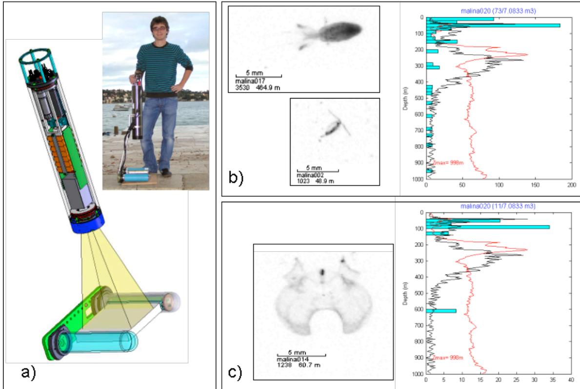
Figure 1: a) UVP5, b) specimens and vertical distribution of copepods (blue), particles below 200  $\mu\text{m}$  (black) and particles above 500  $\mu\text{m}$  (red) at station 20 of Malina cruise, c) specimen and vertical distribution of appendicularia (blue), particles below 200  $\mu\text{m}$  (black) and particles above 500  $\mu\text{m}$  (red) at station 20 of Malina cruise.
