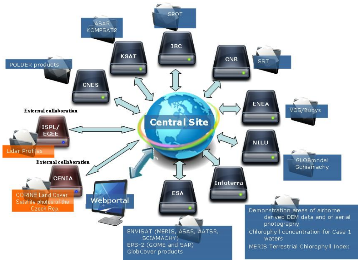
Figure 1. A registered user has direct access to the federated digital repositories (DR's) through the GENESI-DR Central Site. Note the data remain at the federated digital repositories and are not copied to the Central Site, and the individual data DR's policies being respected.
