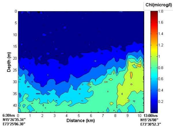
Figure. 2 A depth section of chlorophyll, measured by the AVP from the ship drift over a distance 10kms. In this period the AVP executed 48 dives to 50m every 5mins from 6:30am to 13:00hrs on the 30 April 2009. The profile were used to make the curtain plot
