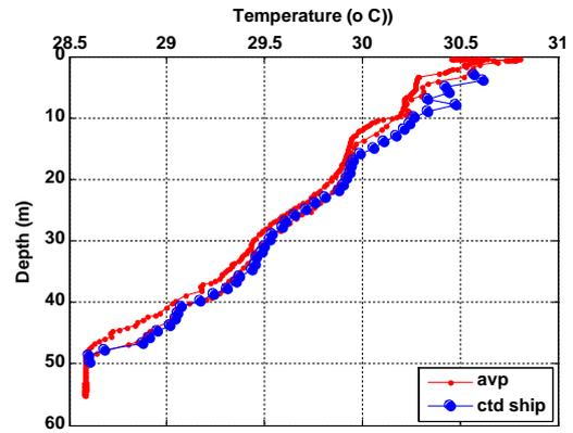
Figure.3 A comparison of the temperature profiles from the AVP CTD sensor and the Seabird CTD on the ship. The small offset is due to a calibration offset on the depth sensor of the ship's CTD.
