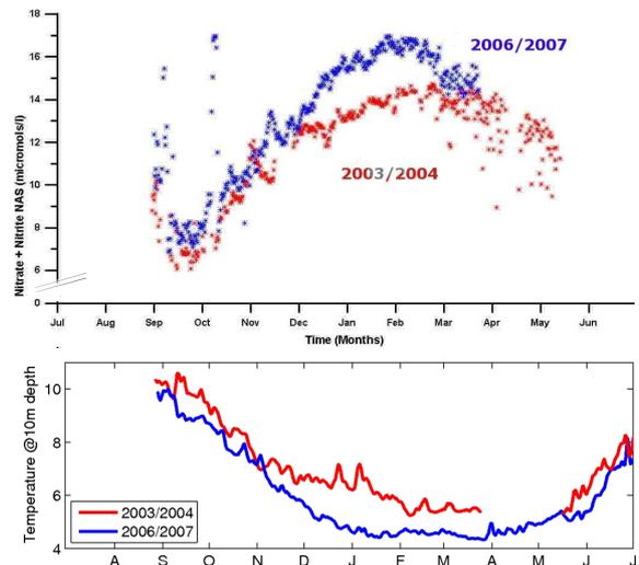
Figure 2: Temporal evolution of the mixed layer nitrate concentration (upper panel) for the years 2003/2004 (red) and 2006/2007 (blue). Note the difference in surface nitrate during the winter month. Scale starts with  $8 \mu\text{mol/l}$ . The temperature at 10m depth (lower panel) also indicates the difference in convection activity – warmer water, less intense convection and lower nitrate values in 2003/2004 and the contrary for 2006/2007.
