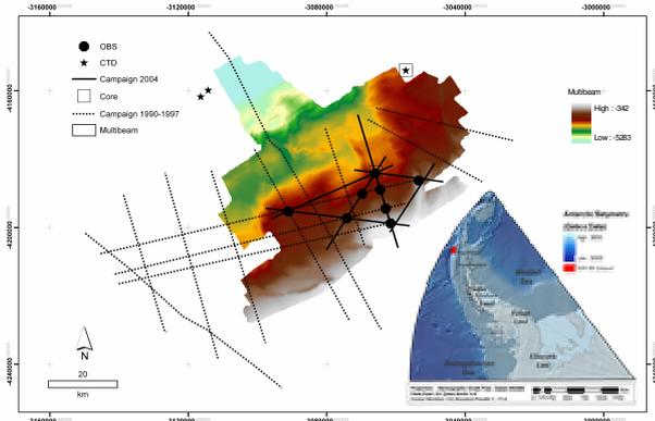
Figure 1. Map showing the locations of the study area, airgun seismic lines acquired in 2004 (continuous lines, present study), 1990 and 1997 (dotted lines, cf. Tinivella and Accaino 2000). CTD measurements (stars), the two coring sites (square), and the border of the Multibeam survey are reported (modified after Tinivella et al. 2007). The Mercator projection with standard parallel equal to 61°S and spheroid WGS84 was adopted.
