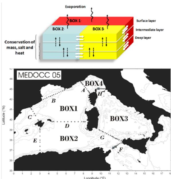
Figure 2. (a) Box model scheme and (b) definition of real boxes using data of a cruise in the Western Mediterranean [3]
