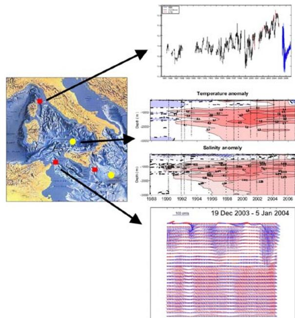
Figure 1. Location of moored chains (red squares) and sites of special interest (yellow circles). Examples of data collected: time series of potential temperature in the Corsica Channel (moored instruments since 1985), T and S anomalies in the central Tyrrhenian basin (repeated CTD casts since 1988), current profiles in the Sicily Strait (moored instruments since 1994).
