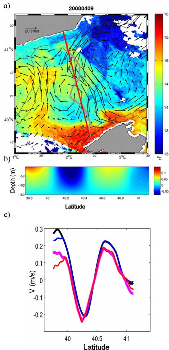
Figure 1. Results of a glider mission (April 2008) along an ENVISAT track in the Balearic Sea. a) Synoptic view
