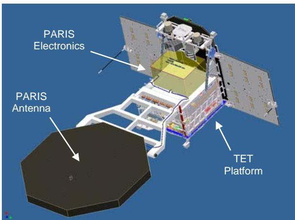
During launch, the antenna is folded with the array sitting flat on top of the platform. The required deployment is performed in two steps through two parallel hinge lines. The electronics of the PARIS altimeter are housed on top of the thermal interface
