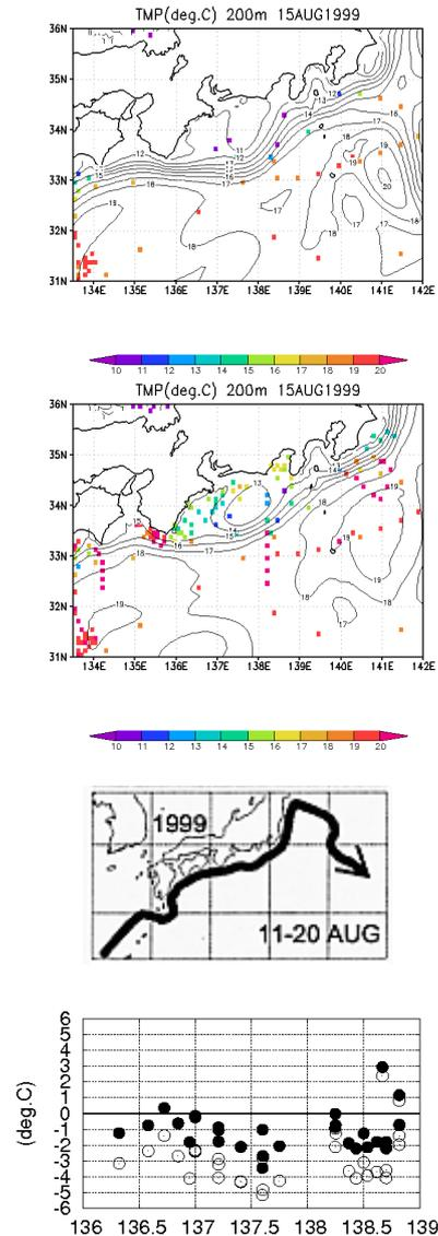
Fig.2: Upper: Contours (colored squares) denote reanalysis (observed) temperature of 200m depth. Upper: noFRA with GTSP. Upper middle: FRA-JCOPE2 with GTSP+VOD+FRA. Lower middle: Observed Kuroshio path from 11 to 20 August 1999 reported by Japan Meteorological Agency. Lower: Biases of temperature profiles in  $34^{\circ}$  -  $35^{\circ}\text{N}$ ,  $136^{\circ}$  -  $139^{\circ}\text{E}$  for FRA-DATA. 'FRA' denotes FRA-JCOPE2.
