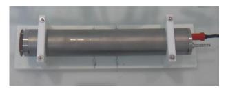
Figure 1. HydroC<sup>TM</sup>/CO2 within a POM mounting. The sensor head is on the left. Cable connection and an external temperature probe are on the right end of the tube. The titanium housing is 90 mm in diameter and sensor has an overall length of 550 mm.
