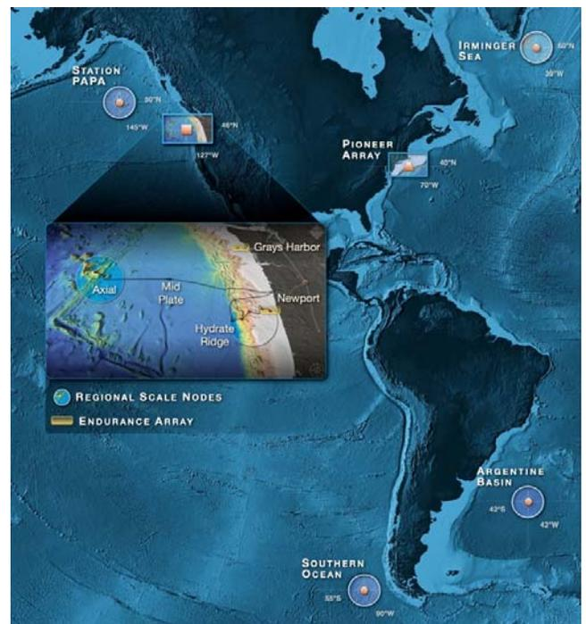
Figure 2. Geographic locations of the components of the OOI, including global moorings in mid and high latitude regions, coastal observatories on the West and East Coasts, and regional cabled nodes on a tectonic plate off the coast of the Pacific Northwest.
