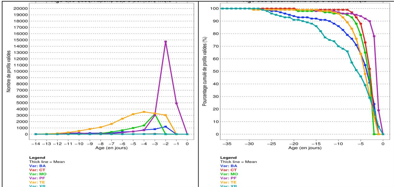
Figure 1 : Statistics of in-situ data provided by the Coriolis data centre and processed at CLS between April and June 2009. Left : age of data by type (PF, profilers / BA, Global Transmission System [GTS] BATHY messages / CT, CTDs / MO, moorings / TE, GTS TESAC messages / XB, XBTs). Right : cumulated number of data per type (courtesy of Mercator-Océan).
